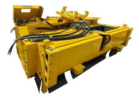
Due to its compact dimensions and the adjustable height of the rollers, the SB1 Ballast Broom can be used for any kind of track. The SB1 can be used on either concrete or wooden ties. In addition, the direction of the ballast conveyor belt can be switched from right to left from by the excavator operator.
