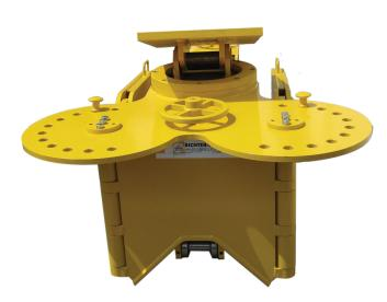
Due to its compact dimensions and adjustable guide rollers, and applicable to concrete or wooden ties, the S1 Ballast Plow can be used under any track conditions., A simple adjustment of the side panels permits you to shift ballast from left to right and vice versa, eliminating time consuming ballast transfer operations using a bucket or grapple.
