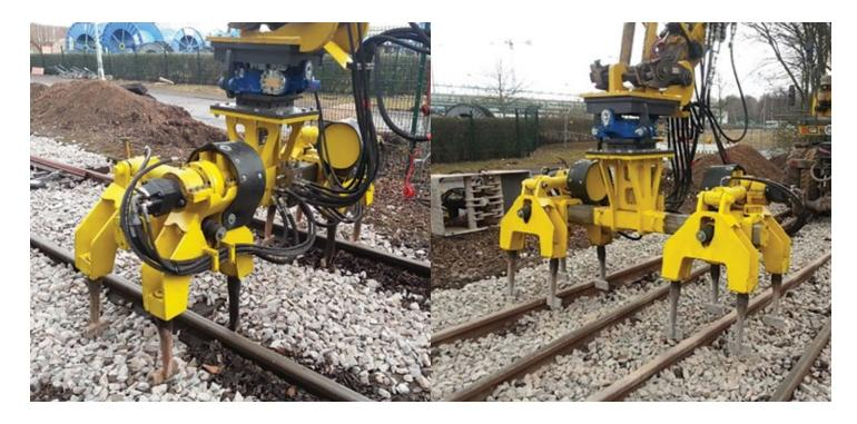
The twin bank tamper is designed as a boom mounted system special for road-rail excavators. Applications of the MSG 8 are mostly small and middle sized working-sites.
