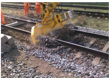
The new HSW2 hydraulic tie changer is a multifunctional unit with removable bucket components to excavate ballast and change single ties.
