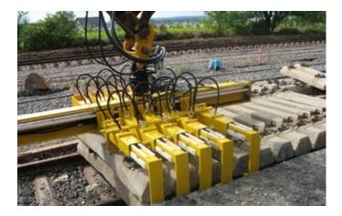
This hydraulic tie spreading device is a multifunctional tool to efficiently unload and lay wooden and concrete ties. Working together with an excavator, the HSG 5 can rapidly pick up, spread, and lay 5 ties.
